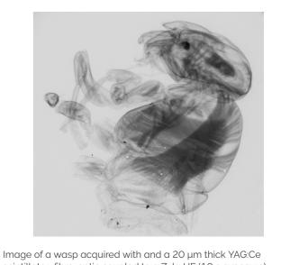
scintillator fibre-optic coupled to a Zyla HF (10 s exposure) X-ray source Cu target, 40 keV, 2 W Image courtesy of Crytur
