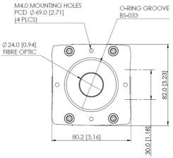
1.3 ±0.5 FIBRE OPTIC PROTRUSION 45.2 [1.78] 159.1 [6.26]
